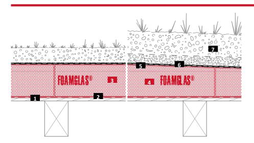
1 Timber deck / multilayer composite board 2 Separating layer nailed on or self-adhesive layer
