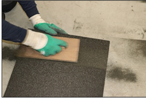
Abrading the bottom side
