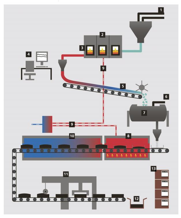
1 Mixing and batching of the raw materials: Recycled glass, feldspar, sodium carbonate, iron oxide, manganese oxide, sodium sulphate, sodium nitrate. 2 The melting furnace has a constant temperature of 1250°C.
