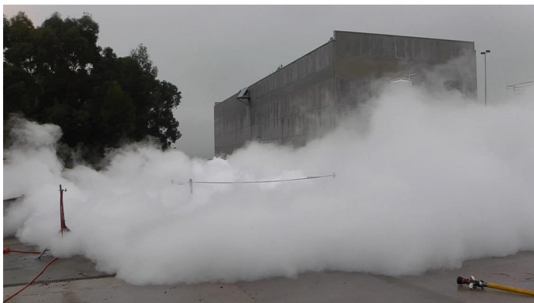
Figure 9: LNG is released into the test pit and gas concentration is measured
