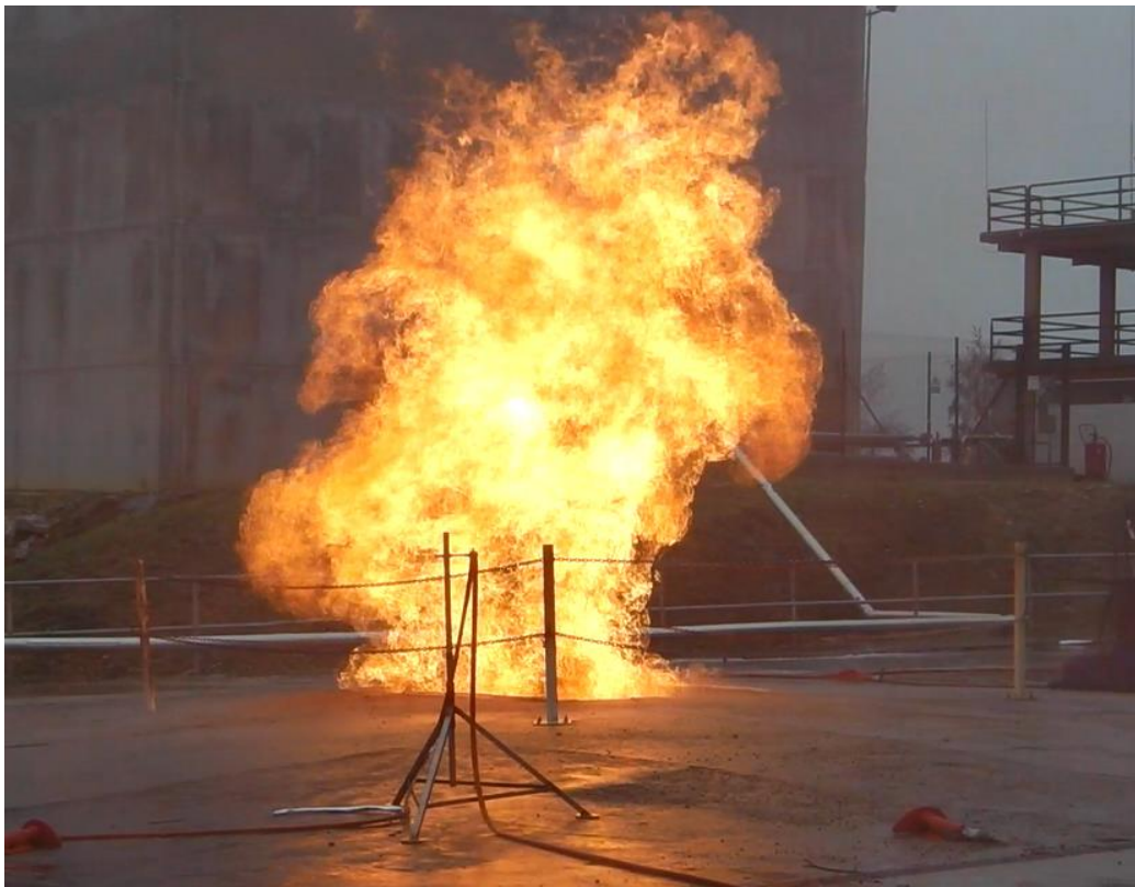
Figure 12: Radiant heat being measured during the LNG pool fire reference test (test 1)
