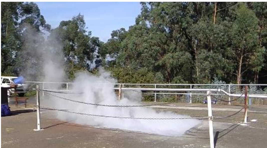
Figure 15: LNG vapour, after moving the discharge line
