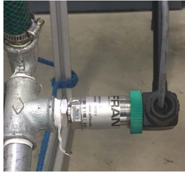
b) Pressure gauge (Gefran TK-E-1-E-B16U-H-V with accuracy \pm 0.25\% FSO) for the internal pressure's chamber monitoring.
