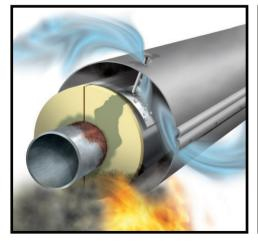
Conventional cold system with plastic foam insulation
