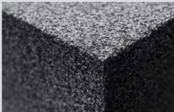
Closed-cell structure of FOAMGLAS® cellular glass.
