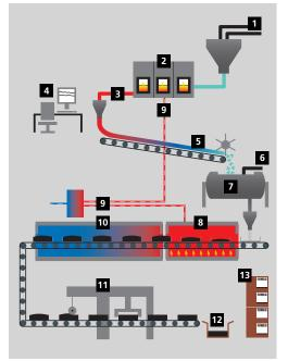
Raw materials and the manufacturing process determine the unique combination of properties of this unusual insulation. First from a fusion of recycled glass, sand, dolomite, lime, iron oxide etc. a glass with precisely defined properties is obtained. In a further part of the process the glass is ground, mixed with a small amount of carbon and put in high-grade steel moulds. The moulds then pass through a furnace in which the glass foam powder is expanded.
