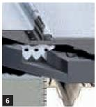
Fully supported standing seam roofing. Aluminium roofing, 6
