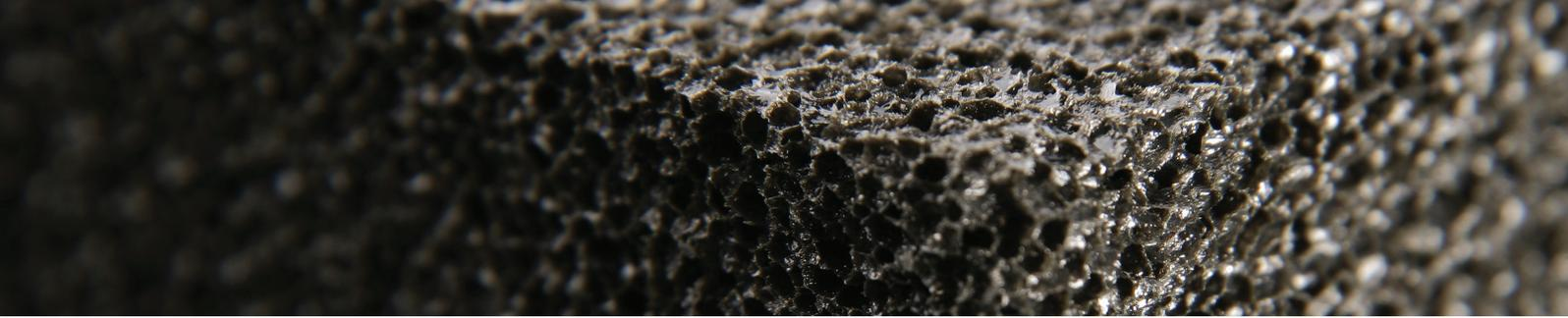
The temperature at which this condensation begins is called the *dew point*. As we will see, the existence of vapor pressure differences, particularly under humid conditions, is the nemesis for permeable insulation on chilled water systems.
