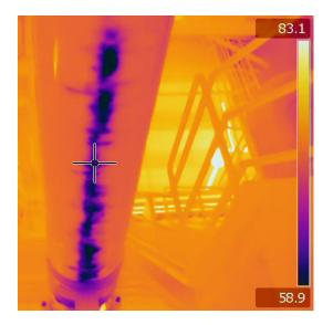
Furthermore, the impact of moisture intrusion does not end with the degradation of insulation and chilled water system efficiency. Moisture intrusion is the common denominator in other effects including surface sweating, mold and mildew formation, as well as a likely increase in the corrosion of pipes, fittings, hangers, etc.
