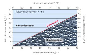
This inward passage of water driven by vapor pressure differences develops any time the cold/low-temperature or chilled water system (normally at 4.4°C to 7.2°C (40°F to 45°F) operates below the local dew point, which for humid coastal areas is a regular condition. As the dew point temperature increases, the vapor pressure of saturated air increases; and, as the operating temperature and the dew point increase, the vapor pressure drive into the system insulation also increases.
