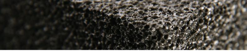
The high strength to weight ratio of FOAMGLAS<sup>®</sup> insulation makes it ideal for suspended chilled water lines and allows it to withstand physical abuse and loads.
