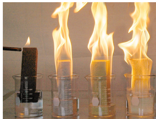
Wicking test with calcium silicate, microporous silicate and perlite.
