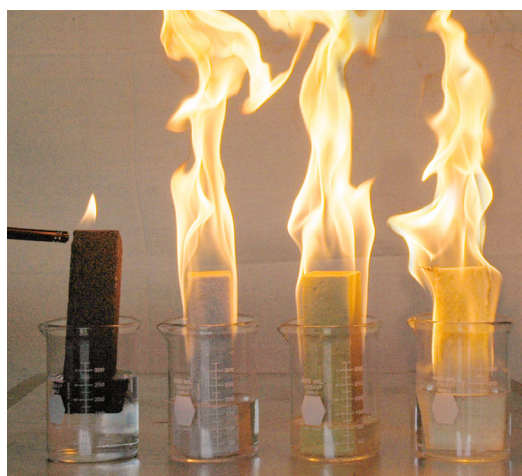
Wicking test with calcium silicate, microporous silicate and perlite.
