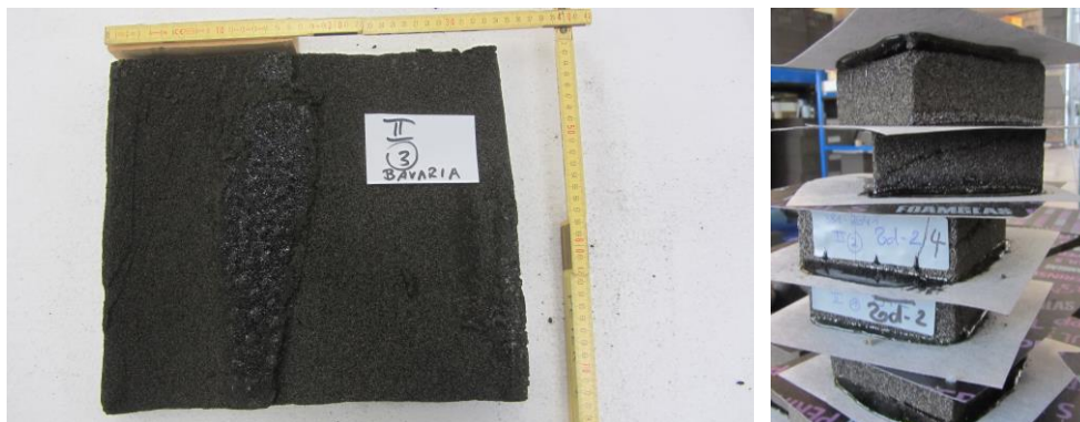
Figure 3: Sample (1 out of 4) as arrived in the FIW laboratories (left), specimens for measurement of compressive strength (already tested) (right).
