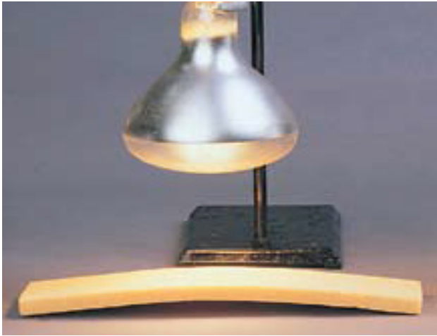
Warping of polyisocyanurate under the influence of temperature.
